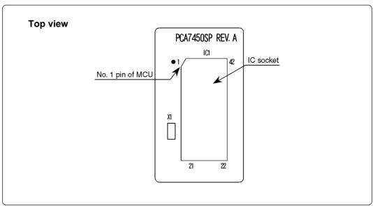
Figure 4.4 Mounting an MCU (PCA7450SP)
