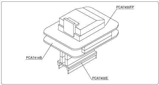
Figure 2.1 External view of the PCA7450FP and its constituent parts
