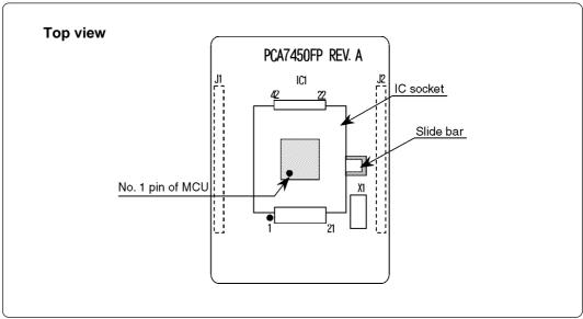
Figure 4.3 Mounting an MCU (PCA7450FP)
