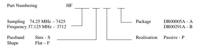
Example part number HF7425SPA is a passive, luminance, sinx/x corrected for a S.F. of 74.25 MHz packaged in a 11 pin SIL as DR00005A
