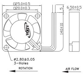
Frame:Plastic(UL:94V-0) Impeller:Plastic(UL:94V-0) Lead wire:UL1571AWG28
