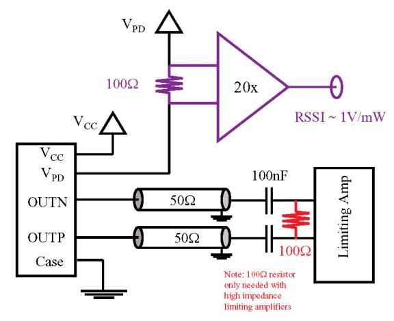
Optional 100 $\Omega$  differential termination for high impedance limiting amplifiers is shown in red
