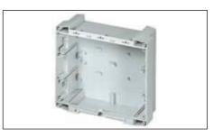
**UT:** All bases have plug-in slots and fixing domes for circuit boards, mounting panels or DIN rails. As an option, a variable terminal compartment can be integrated and isolated from the electronics compartment. The external surfaces have no pre-punchings, so individual arrangement of cable entries or connections is possible. Depending on the installation side which is used, fitted cable glands are partially concealed.
