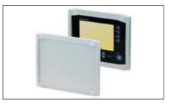
**CF:** The installation area has a recessed section for mounting membrane keypads. It can be screwed to a rear panel with four screws. Ingress protection IP 65 to the installation front can be achieved with the optional seal. Cannot be combined with Bocard bases.
