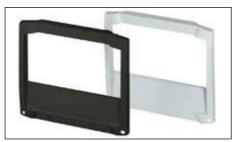
**FO-K:** The FO-K frame is used for edge covering of a front panel (FP...K) and a terminal compartment. The integrated terminal compartment lid has a 1.5 mm recessed area for the fitting of membrane keypads. The frame is pushed onto the base, pressed tight in 2 places, and screwed to the terminal compartment. In connection with base and front panel: protection class IP 40.
