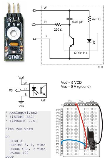
When W is connected to Vdd and B is connected to Vss, the R terminal's voltage will drop below 1.4 V when the IR transistor sees infrared reflected from the IR LED. When the IR LED's signal is mostly absorbed by a black surface, the voltage at R goes above 1.4 V. Since the BASIC Stamp interprets any voltage above 1.4 V as 1 and any voltage below 1.4 V as 0, this circuit gives us a quick and easy way to detect a black line on a white background.
