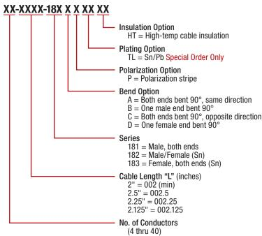
NOTE: Please contact the factory for price and availability of any high-temp (HT) cable larger than 20 conductors.
