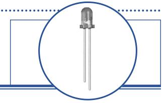
The OPV332 is a Vertical Cavity Surface Emitting Laser (VCSEL) packaged in a dome lens T-1 package. VCSELs offer many advantages in sensing applications when compared to infrared LEDs. These devices require substantially lower drive currents to obtain the same amount of output power as LEDs. This feature allows VCSELs to be used in low power consumption applications such as battery operated equipment.
