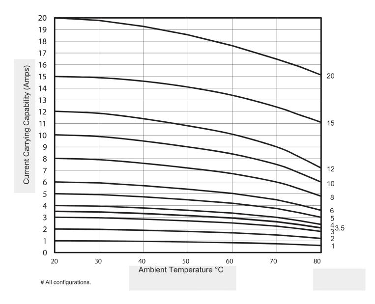
No additional derating is required for PV fuse links installed in ganged modular fuse holders without spacing between units, provided that the rating used is  $>1.56 \times I_{sc}$ .
