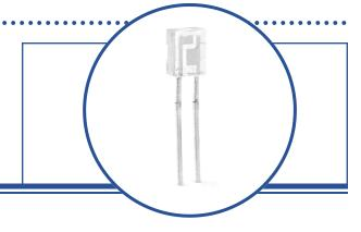
The OPV380 is a Vertical Cavity Surface Emitting Laser (VCSEL) packaged in a flat lens lateral package. VCSELs offer many advantages in sensing applications when compared to infrared LEDs. These devices require substantially lower drive currents to obtain the same amount of output power as LEDs. This feature allows VCSELs to be used in low power consumption applications such as battery operated equipment.
