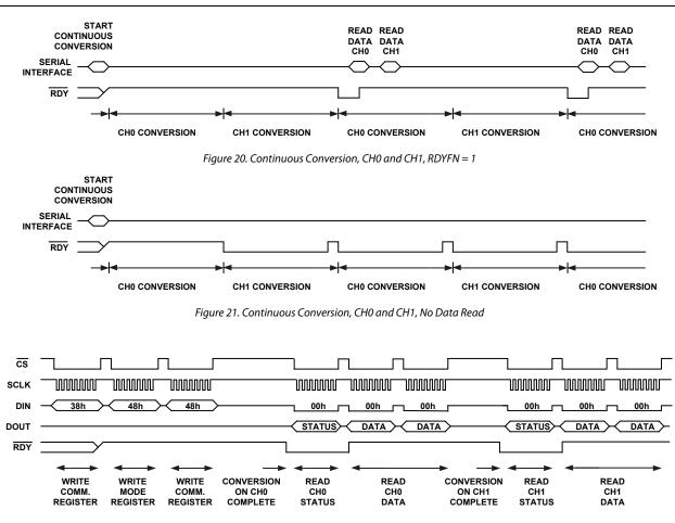
Figure 22. Continuous Conversion, CH0 and CH1, Continuous Read
