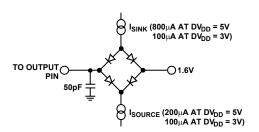
Figure 4. Load Circuit for Access Time and Bus Relinquish Time
