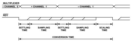
Figure 25. Multiplexer and Conversion Timing—Continuous Conversion on Several Channels with Chopping Enabled
