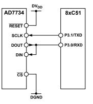
Figure 15. AD7734 to Host Device Interface, 2-Wire Configuration
