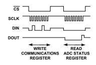
Figure 16. Serial Interface Signals—Registers Access
