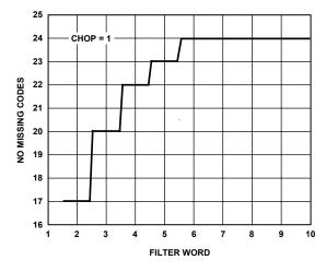
Figure 5. No Missing Codes Performance, Chopping Enabled
