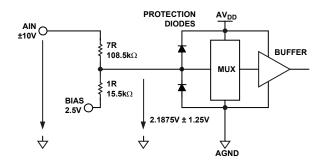
Figure 23. Simplified Analog Input Internal Structure
