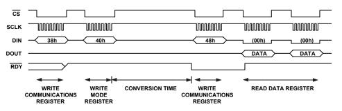
Figure 17. Serial Interface Signals—Single Conversion Command and 16-Bits Data Reading
