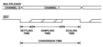
Figure 26. Multiplexer and Conversion Timing—Continuous Conversion on Several Channels with Chopping Disabled
