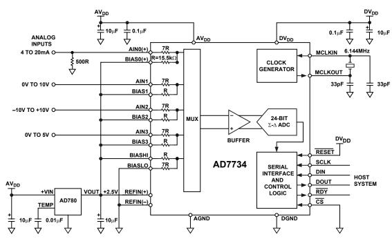
Figure 29. Typical Connections for the AD7734 Application
