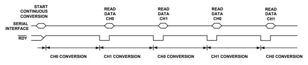
Figure 19. Continuous Conversion, CH0 and CH1, RDYFN = 0
