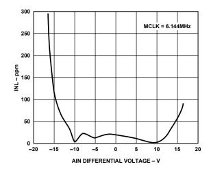
Figure 8. Typical INL vs. AIN Voltage, AIN Range = $\pm 10 V$ , BIASO to BIAS3, BIASHI = 2.5 V, BIASLO = O V
