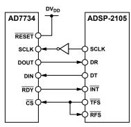
Figure 14. AD7734 to Host Device Interface, DSP
