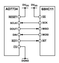
Figure 13. AD7734 to Host Device Interface, SPI
