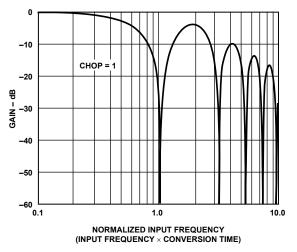
Figure 28. Typical ADC Frequency Response, Chopping Disabled
