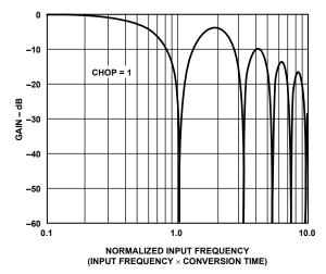
Figure 27. Typical ADC Frequency Response, Chopping Enabled
