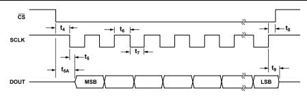
Figure 2. Read Cycle Timing Diagram
