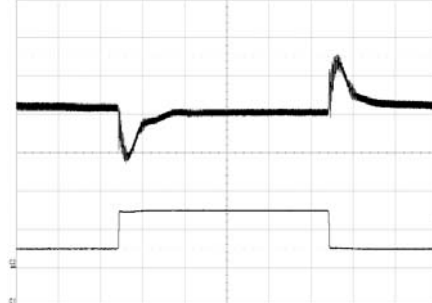
Output voltage response to load current step- change (5 - 15 - 5 A) at: T_{ref} = +25^{\circ}C, V_1 = 53 V, C_o = 2.2mF
