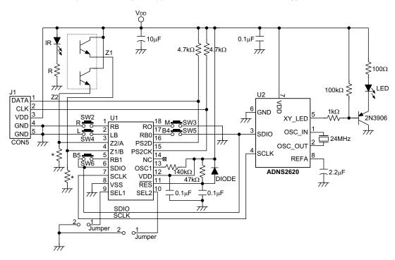
Note: \* For resistor value selection, refer to high or low input level of Z1 and Z2 in the D.C. Characteristics table. The recommended value is  $6k\Omega$ .
