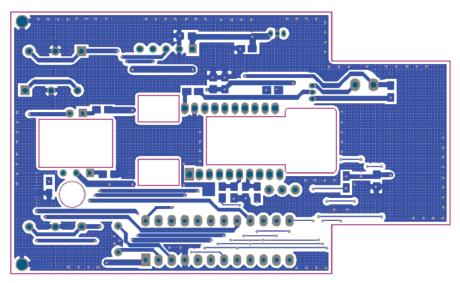
Figure C1: PCB Schematic (Bottom Layer)
