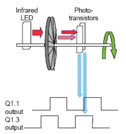
Figure 2. Optics Quadrature Signal Generation
