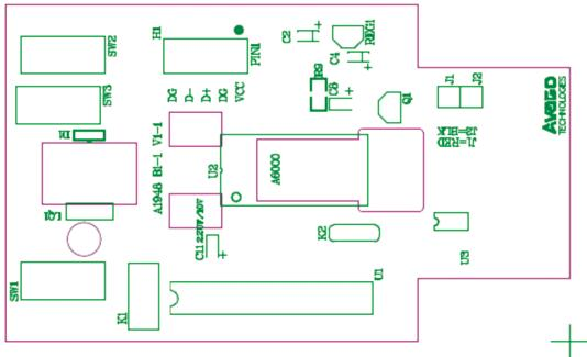
Figure C3: PCB Schematic (Top Overlay)
