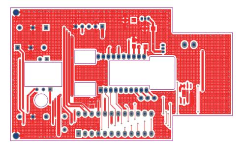
Figure C2: PCB Schematic (Top Layer)
