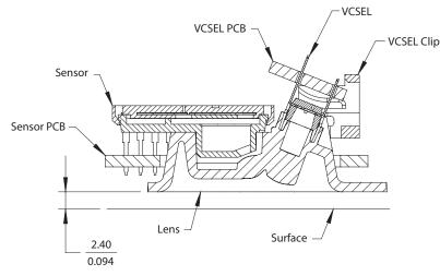
Figure 5. Distance from lens reference plane to surface
