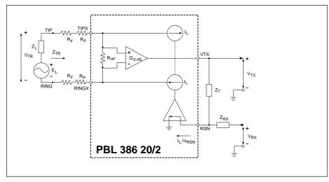
Figure 9. Simplified ac transmission circuit.
