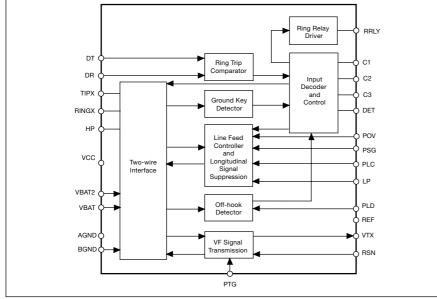
The PBL 386 20/2 Subscriber Line Interface Circuit (SLIC) is a 90 V bipolar integrated circuit for use in PBX.Terminal adapters and other telecommunications equipment.
