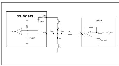
Figure 14. CODEC receive interface.
