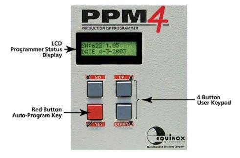
In 'Standalone Mode', the programmer is controlled via the push buttons on the front panel of the programmer - no PC connection is required. The programmer LCD and the LED Status Indicators are used to display the current status of the programmer. It is possible to select from 1 of 64 previously uploaded 'Programming Projects' and then to repeatedly execute this project by pressing the [YES] button to program a batch of devices.
