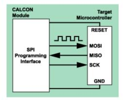
The PPM4-MK1 programmer can be used to perform a very accurate Calibration (+/1 1%) of the Internal Oscillator of many Atmel AVR microcontrollers. This requires the use of the 'EQ-SFM-MAX-V1.3' module.
