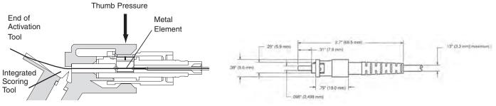
The metal element inside the connector closes around the fiber.
