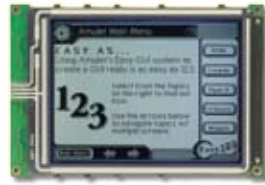
MK-AOB3202405N (FSTN Negative, Transmissive)
