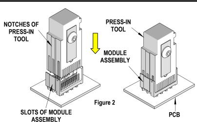
3. Using the application tool and an appropriate press, seat the header assembly until there is less than 0.10mm (.004 in) clearance between the bottom of the plastic housing and the surface of the PCB. See Figure 3.
