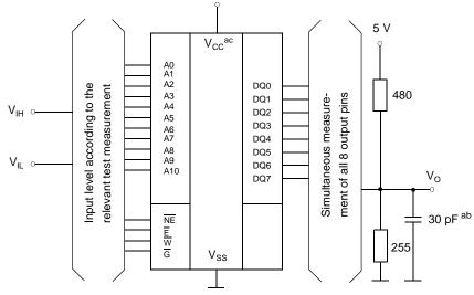
ab: In measurement of  $t_{dis}$ -times and  $t_{en}$ -times the capacitance is 5 pF.
