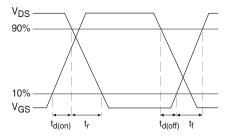
Fig 18b. Switching Time Waveforms
