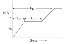
Fig 13a. Basic Gate Charge Waveform
