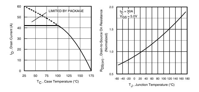
**Fig 9.** Maximum Drain Current Vs. Case Temperature
