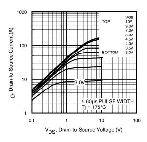
Fig 1. Typical Output Characteristics
