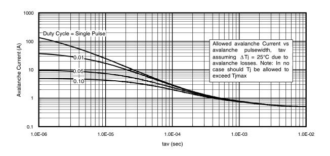
Fig 15. Typical Avalanche Current Vs. Pulsewidth
