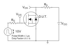
Fig 18a. Switching Time Test Circuit
