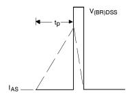
Fig 12b. Unclamped Inductive Waveforms
