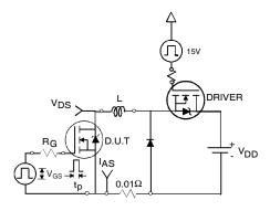
Fig 12a. Unclamped Inductive Test Circuit
