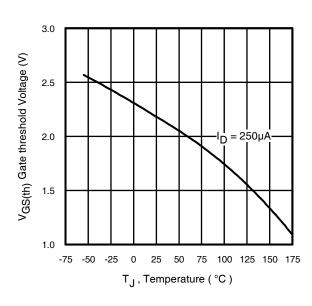
Fig 14. Threshold Voltage Vs. Temperature
