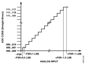
Figure 22. ADC Ideal Transfer Function
