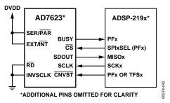
Figure 42. Interfacing the AD7623 to SPI Interface
