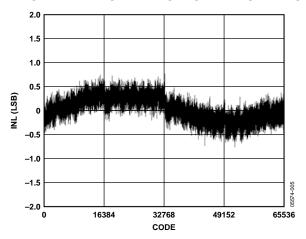
Figure 5. Integral Nonlinearity vs. Code
