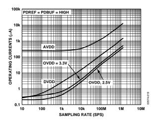
Figure 19. Operating Currents vs. Sample Rate
