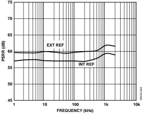
Figure 29. PSRR vs. Frequency
