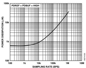
Figure 30. Power Dissipation vs. Sample Rate
