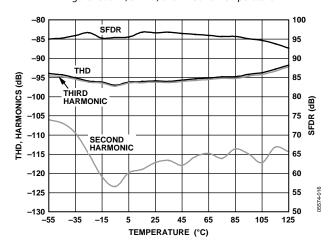
Figure 16. THD, Harmonics, and SFDR vs. Temperature
