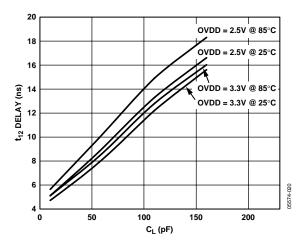
Figure 20. Typical Delay vs. Load Capacitance C<sub>L</sub>
