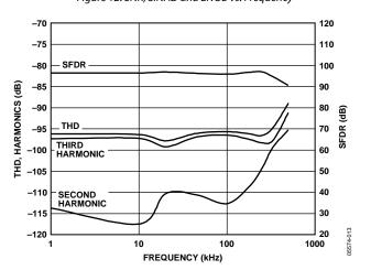
Figure 13. THD, Harmonics, and SFDR vs. Frequency
