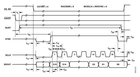
Figure 37. Master Serial Data Timing for Reading (Read After Convert)
