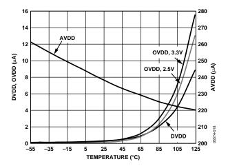
Figure 18. Power-Down Operating Currents vs. Temperature
