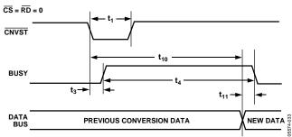
Figure 33. Master Parallel Data Timina for Reading (Continuous Read)
