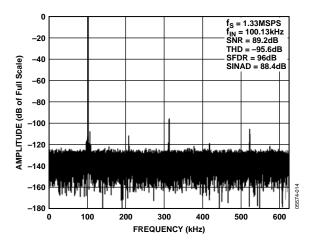
Figure 14. FFT 100 kHz
