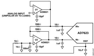
Figure 27. Single-Ended-to-Differential Driver Circuit (Internal Reference Buffer Used)
