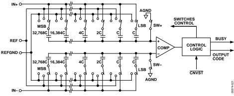
Figure 21. ADC Simplified Schematic
