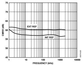
Figure 25. Analog Input CMRR vs. Frequency
