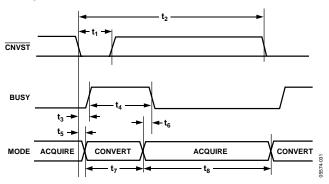
Figure 31. Basic Conversion Timing
