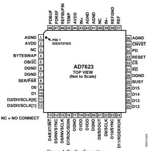
Figure 4. Pin Configuration
