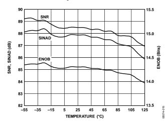
Figure 15. SNR, SINAD, and ENOB vs. Temperature
