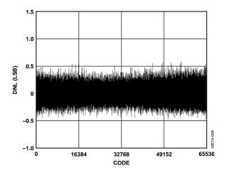
Figure 8. Differential Nonlinearity vs. Code
