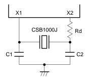
Caution The oscillation circuit constants and oscillation voltage range indicate conditions for stable oscillation, but do not guarantee oscillation frequency accuracy. If oscillation frequency accuracy is required for actual circuits, it is necessary to adjust the oscillation frequency of the resonator in the circuit. Please inquire directly to the maker of the resonator for data as needed.
