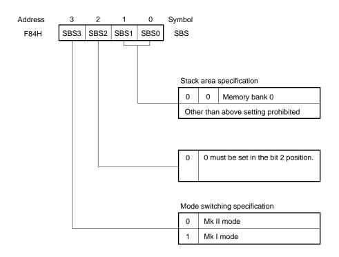
Figure 4-1. Stack Bank Select Register Format
