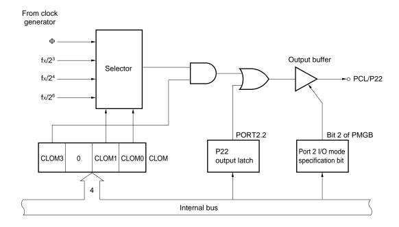
**Remark** Special care has been taken in designing the chip so that small-width pulses may not be output when switching clock output enable/disable.
