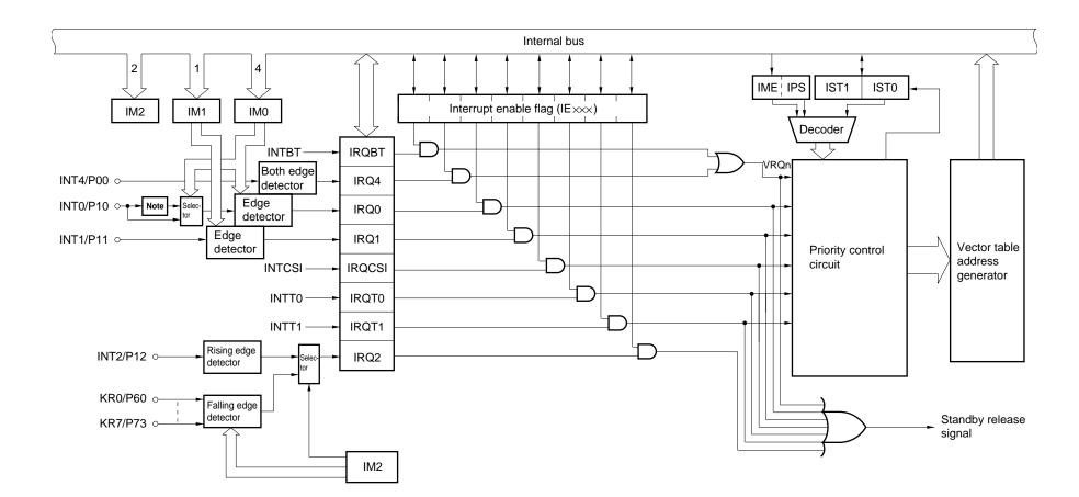
Figure 7-1. Interrupt Control Circuit Block Diagram
