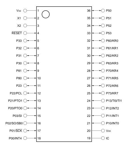
IC: Internally Connected (Connect directly this pin to VDD.)
