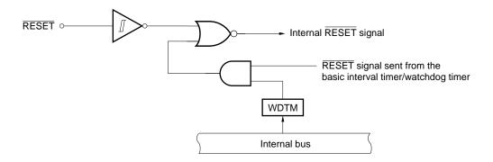
Generation of the RESET signal initializes each hardware as listed in Table 9-1. Figure 9-2 shows the timing chart of the reset operation.
