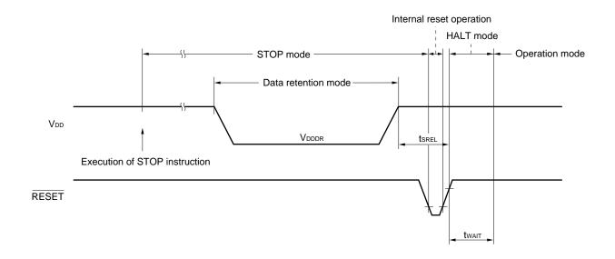
**★** Data Retention Timing (Standby release signal: on releasing STOP mode by interrupt signal)
