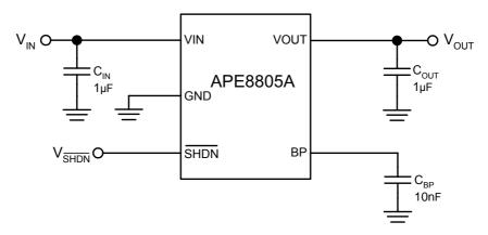
Figure 2. Typical Application Circuit of APE8805A
