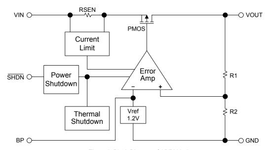
Figure 3. Block Diagram of APE8805A
