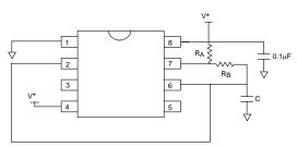
Frequency f = 1.46 / (RA + 2RB)C Duty Cycle DC = RB / (RA + 2RB)
