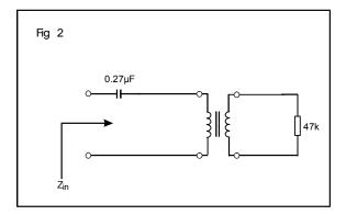
In practice, the 47k $\Omega$  load can be increased without limit. The DC blocking capacitor should be maintained within the range 0.22 $\mu$ F to 0.33 $\mu$ F to obtain a flat frequency response and input impedance to specification.
