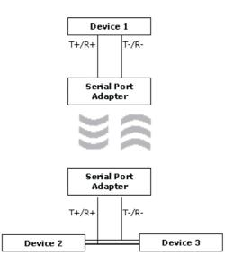
Picture 13. Two-wire RS485 connection setup
