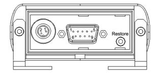
Picture 9. DSUB serial connector (male).
