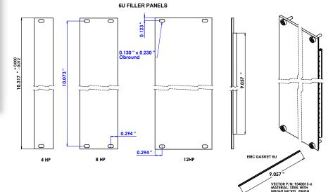
Typical slot width is 0.800" (4HP) Material: 6063T5, extruded brushed Aluminum with clear Chem-Film finish Each Filler Panel Kit Includes 4,8 or 12HP EMC panel with EMC gasket M2.5 Nickel plated mounting screws with 'captive' sleeves
