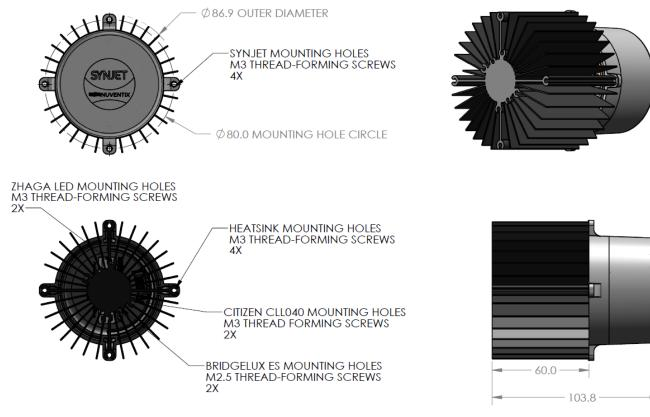
NOTE: DIN 7500 TYPE THREAD-FORMING SCREWS ARE RECOMMENDED FOR ALL MOUNTING HOLE BOSSES
