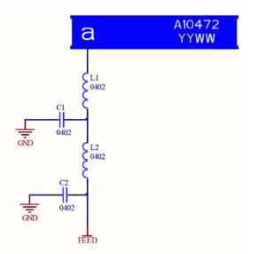
Note: The component values for the matching circuit will vary depending on the size of the PCB and surrounding components. The impedance of the antenna should be measured before selecting suitable matching components. Antenova M2M offers this service on request. Contact sales@antenova-m2m.com for further information.
