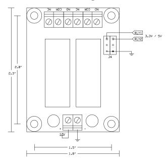
Note: The two pins at the J4 (pins 5/6) label are both ground pins, while the pins labeled RLY1 and RLY2 (pins 1/2) are the signal/control pins. Pins 3 and 4 are no connected but allowed you to connect a powered servo cable without a conflict with the servo supply.
