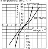
9. Off state leakage current Measured portion: between terminals 3 and 4; Ambient temperature: 25°C 77°F
