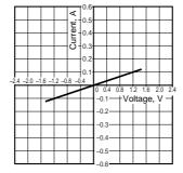
9. Off state leakage current Measured portion: between terminals 5 and 6, 7 and 8; Ambient temperature: 25°C 77°F
