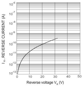
Fig.1 Reverse current Vs. Reverse voltage
