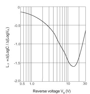
Fig.4 Linearity factor Vs. Reverse voltage
