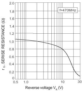
Fig.3 Series resistance Vs. Reverse voltage
