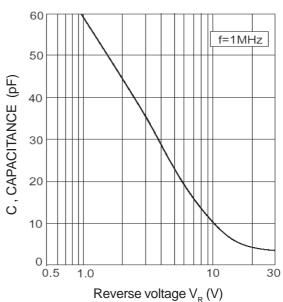
Fig.2 Capacitance Vs. Reverse voltage
