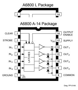
Note: The A6800 SOIC and DIP packages are electrically identical and share a common terminal number assignment.
