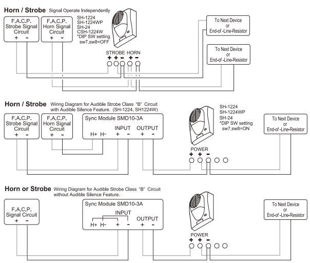
Refer to the SMD 10-3A Sync Module instruction manual for Class "A" wiring or other application diagrams.
