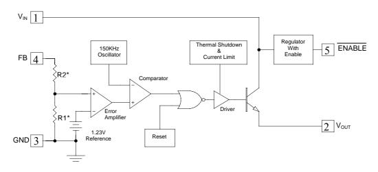
$V_{OUT} = 3.3V$  : R2/R1 = 1.7  $V_{OUT} = 5.0V$  : R2/R1 = 3.1  $V_{OUT} = \text{Adjustable}$  : R2 = 0, R1 = Open
