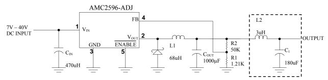
Figure 3. LC Filter for Low Output Ripple
