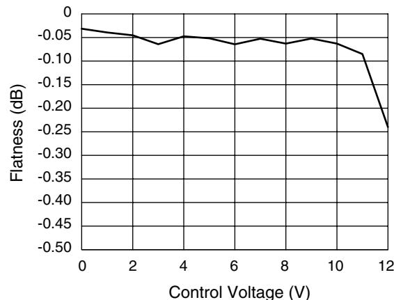
**Insertion Loss Flatness vs. Control Voltage — AMPS Band**
