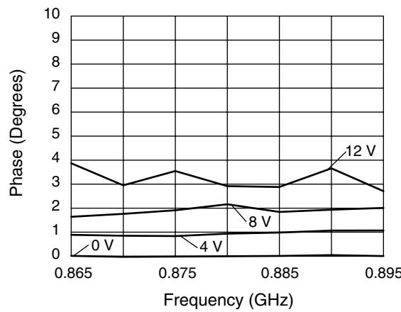
**Phase vs. Frequency and Control Voltage — AMPS Band**
