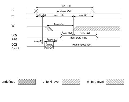
i: If  $\overline{W}$  is LOW and when  $\overline{E}$  goes LOW, the outputs remain in the high impedance state.
