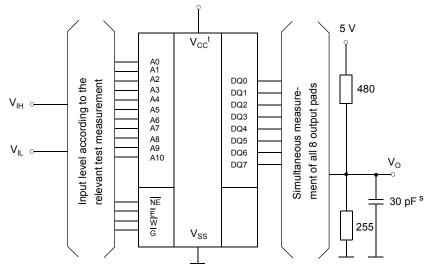
s: In measurement of  $t_{\text{dis}}\text{-times}$  and  $t_{\text{en}}\text{-times}$  the capacitance is 5 pF.
