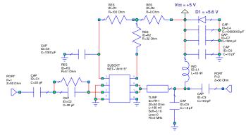
C9 is placed at the silkscreen marker '3' or center of component placed at  $13 \deg$ . @2140 MHz away from pin 6.
