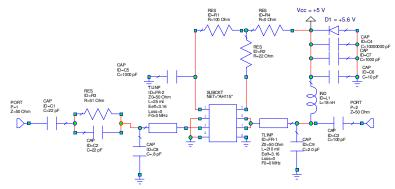
C8 is placed at silkscreen marker 'A' or center of component placed at 1.8 deg. @ 1960 MHz away from pin 3. C9 is placed at the silkscreen marker '4' or center of component placed at 20 deg. @1960 MHz away from pin 6.
