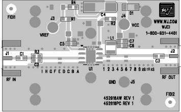
Circuit Board Material: .014" Getek, 4 - layer, 1 oz copper, Microstrip line details: width = .026", spacing = .026" The silk screen markers 'A', 'B', 'C', etc. and '1', '2', '3', etc. are used as placemarkers for the input and output tuning shunt capacitors – C8 and C9. The markers and vias are spaced in .050" increments.
