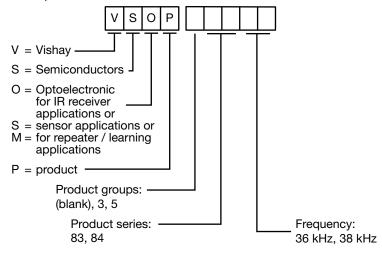
Example: VSOP38336 = receiver chip with f<sub>0</sub> = 36 kHz
