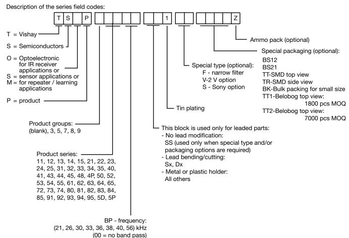
Example: TSOP1236TB1 = receiver with f<sub>0</sub> = 36 kHz, bent in a top view holder, and solder plated leads
