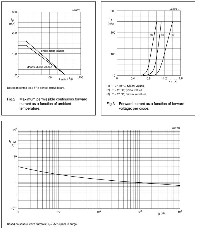
Fig.4 Maximum permissible non-repetitive peak forward current as a function of pulse duration per diode.
