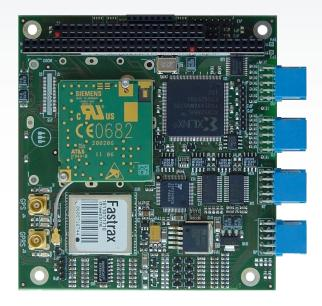
The Eurotech COM-1289 integrates GSM/GPRS (optionally GSM-R) wireless cellular connectivity and a low power GPS receiver within a PC/104 module. This low power integrated telematics board is the ideal choice for onboard computing applications requiring GPRS roaming across three continents and precise GPS positioning. A standard SIM-card can be installed onboard into a locking card holder, or onto an external SIM card carrier.
