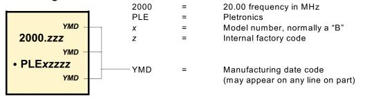
The actual part number is OED4204-10.00M where the model number "204" is the specification number the part is made to. This is not included in the part marking. This is included on the label on the Tape and Reel.
