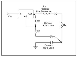
the top of  $R_1$  is internally connected to the output and ground pin can be connected to low side of the load as a negative side sense if, so desired.
