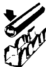
1. Prior to conductor insertion.
