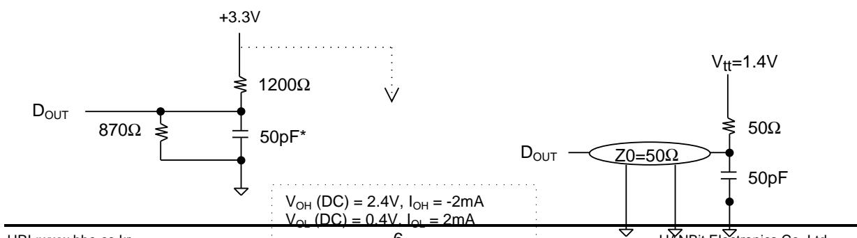
(Fig. 1) DC output load circuit
