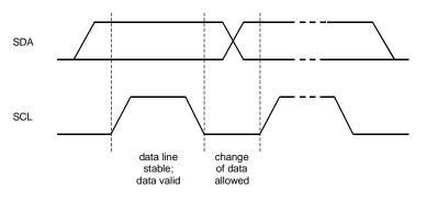
Figure 24. Bit transfer on the I<sup>2</sup>C-bus
