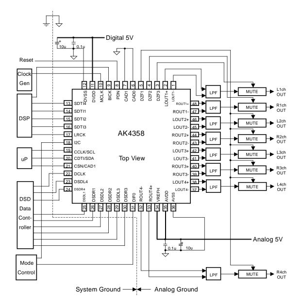
Figure 25. Typical Connection Diagram
