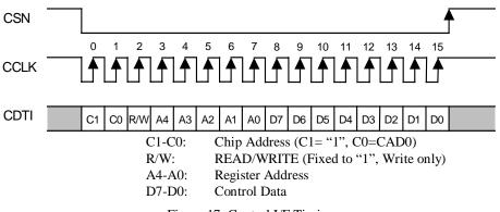
Figure 17. Control I/F Timing
