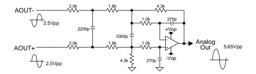
Figure 27. External 3rd order LPF Circuit Example
