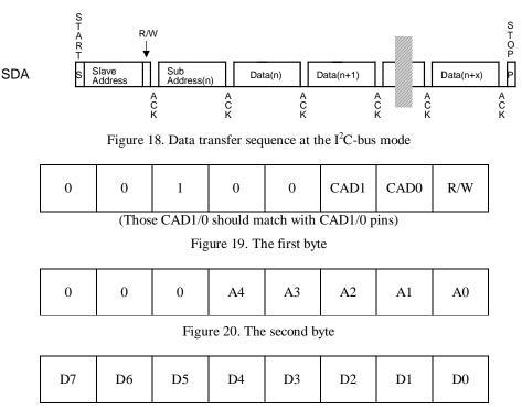
Figure 21. Byte structure after the second byte
