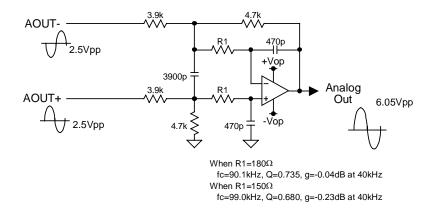
Figure 28. External 2<sup>nd</sup> order LPF Circuit Example for PCM
