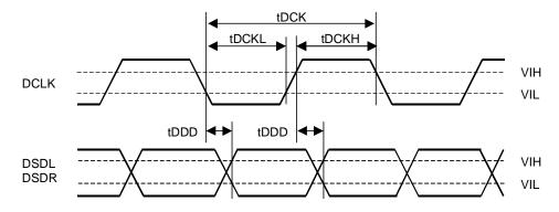
Audio Serial Interface Timing (DSD Phase Modulation Mode, DCKB = "0")
