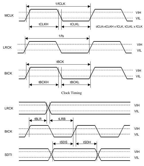
Audio Serial Interface Timing (PCM Mode)
