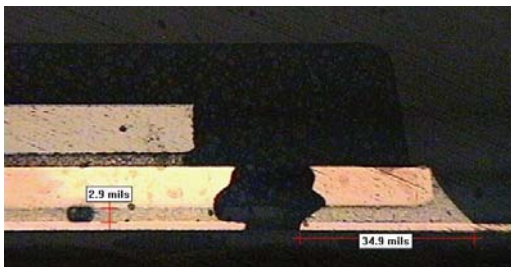
50% Paste Coverage, Plugged Via, 2.9 mil Standoff
