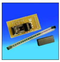
This kit was created to facilitate laboratory experimentation and developed using GMR digital switch output sensors. The kit consists of 16 distinct GMR sensors that span the magnetic field range and output types available in the AD series. All sensors in this kit are packaged in the TSSOP miniature surface mount package. The kit also includes a
